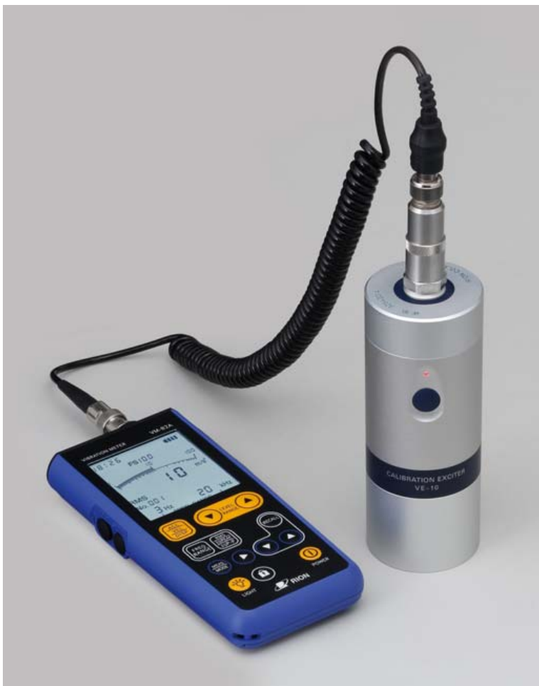
Calibration of Vibration Meter VM-82A by VE-10
