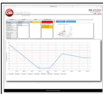
**Trending:** View vibration and temperature trend charts. Colored threshold lines indicate when a measurement has passed user configured vibration threshold limits.
